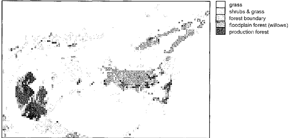
Fig. 3 Vegetation types obtained by classification of the laser altimetry data using the frequency distribution of measured average vegetation heights per 25 \times 25 \text{ m}^2 windows.
